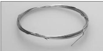
**E436-1** Platin-/Iridium-Draht. 80%/20%, 0,25 mm  $\varnothing$ , 1 m
