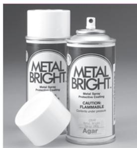
Metal Bright is used for cleaning up after vacuum deposition work. Spray Metal Bright onto the metal surfaces of vacuum deposition equipment, contact masks and shields, and wipe with a damp cloth, cleaning away all water soluble polymer coating plus the deposited materials that have adhered.
