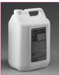
This is a water rinsable, surface active cleaning agent for laboratory cleaning applications. It is phosphate-free and biodegradable. Normal pH in 10 % solution is 13; it will therefore etch certain non-ferrous metals, especially aluminium and zinc. The solution is recommended for glass, plastics, ceramics, rubber, and all ferrous metals. For maximum efficiency, use in an ultrasonic bath.
