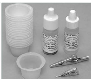
Epoxy Bond 110 is a hard fast curing epoxy adhesive commonly used to bond glass coverslips to small or delicate samples, adhere multiple samples for TEM cross-sections, pre-coat samples prior to encapsulation and for other mounting applications. The two part epoxy cures bubble-free in five minutes at 150 °C (302 °F). Epoxy Bond 110 turns red on curing allowing curing by colour instead of time. Once cured, it is chemically resistant to etchants and will not outgas under vacuum.
