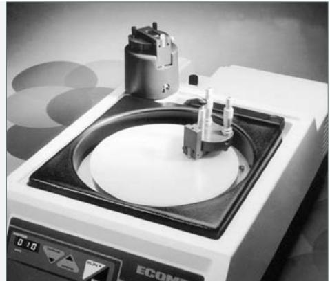
The addition of an Automet power head converts the Ecomet polisher/grinder into a semi-automatic sample preparation system; please ask for details.
