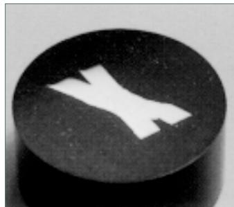
Demotec 70 is a conductive two component resin based on methyl methacrylate and electrically conductive carbon. It has been specially developed for SEM, EDS, microprobe and FIB applications and for electrochemical polishing of samples. It is a two component, black, cold embedding material with graphite added to provide conductivity.
