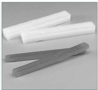
**Crystalbond 509** provides excellent adhesion, and offers reduced clogging of diamond tools compared with waxes. It is transparent in thin cross-sections, and available in two standard colours: amber and clear. It is soluble in acetone or 509-S stripper, an odourless, non-flammable, biodegradable polar solvent.
