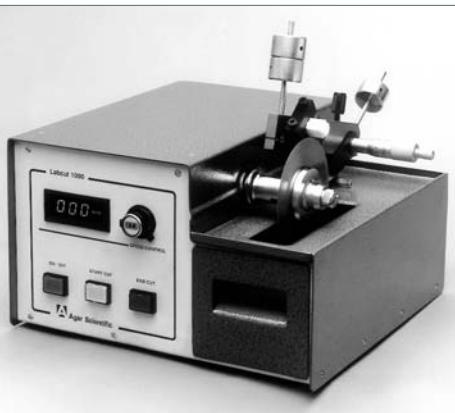
Low speed diamond saws offer convenient, precision cutting for a wide variety of materials in the laboratory, including mineralogical sections, embedded tissue, teeth, bone, semiconductors and other embedded devices. Low speed saws cause minimal damage and deformation of the sample and are particularly suited to fragile or soft materials.
