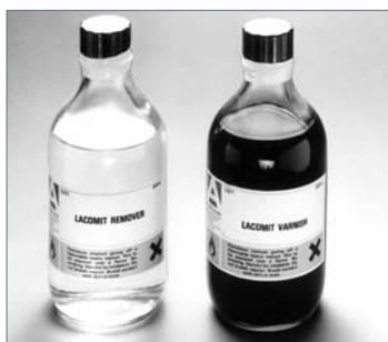
For those who wish to prepare thinned specimens by one of the window techniques, Lacomit peelable varnish is very valuable for blanking off portions of the specimen which are not to be polished. A solvent for the varnish is also available. It may also be used for thinning the varnish consistency if desired.
