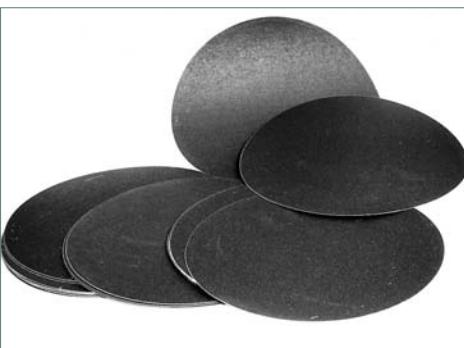
Suitable for most makes of rotary grinders/polishers, these waterproof, self adhesive silicon carbide discs (PSA backed) are available in a range of grit sizes from P60 (269 µm) to P2500 (10 µm). Standard discs are 203 mm (8") in diameter, but other sizes are available.
